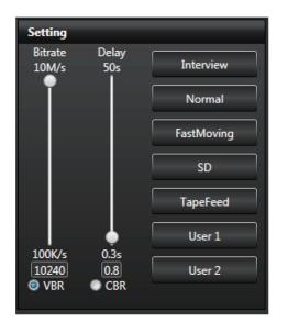
Smart VBR Technology – TVU's Smart VBR functionality enables TVU transmitter devices to adapt quickly and efficiently to extreme fluctuations in bandwidth during live transmissions. The operator only has to set the desired latency for the live shot, and Smart VBR will automatically adjust picture quality based on the available bandwidth.
